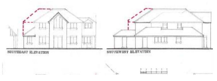
Refused scheme overlaid on proposed SE and SW elevations
